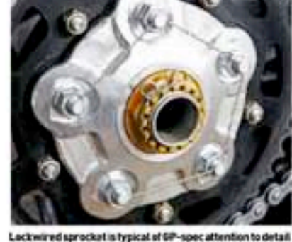
Lock-wired sprocket is typical of GP-spec attention to detail
