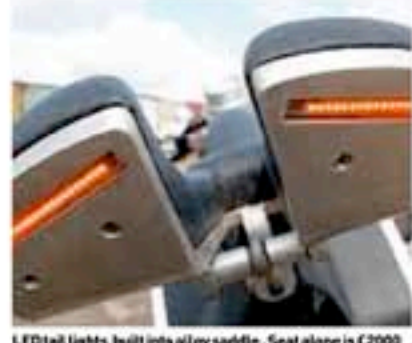
LED tail lights built into alloy saddle. Seat alone is £2000
