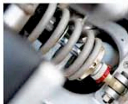
Top-spec, multi-adjustable shocks are by Penske
