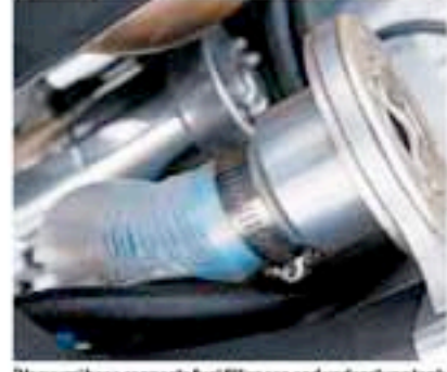
Vacuum hose connects fuel filler cap and under-slung tank
